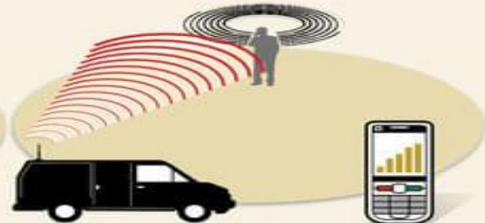
**2.** The stingray system, which mimics a cellphone tower, gets the target phone to connect to it.
