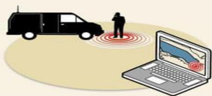
**5.** By collecting signal strength in several locations, the system can triangulate and map a phone's location.
