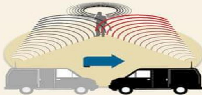
**4.** The vehicle can then move to another location and again measure the phone's signal strength.
